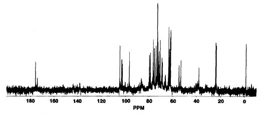
Fig. 1. 75-MHz <sup>13</sup>C NMR spectrum of the O24 polysaccharide, recorded in D<sub>2</sub>O (70°C) with acetone (δ 31.45) as internal standard.
